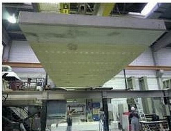
Hoisting the floor at the end of testing and visual inspection - with the exception of minor, superficial spalling, no damage could be detected
