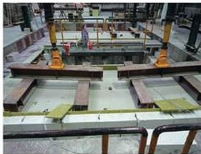
State after 120 minutes – the test floor had yielded 15 cm under the heavy loading and the temperature in the fire testing chamber had risen to 1,034°C
